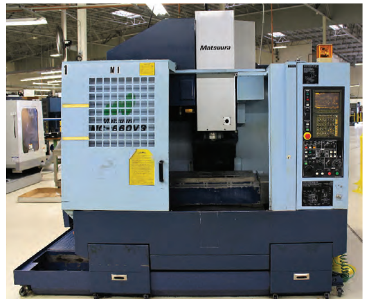
1999 MATSUURA MC-660 VG, YASNAC I-80 CNC CONTROL, TRAVELS: 23" X 16" X 19", 15000 RPM SPINDLE, CAT 40 TAPER, 21 STATION ATC, 10 HP, S/N 990413642
