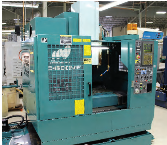
1998 MATSUURA MC-600 VF, YASNAC I-80 CNC CONTROL, 23" X 16" X 18", 8000 RPM SPINDLE, CAT 40 TAPER, 20 STATION ATC, 10 HP, S/N 980713232
