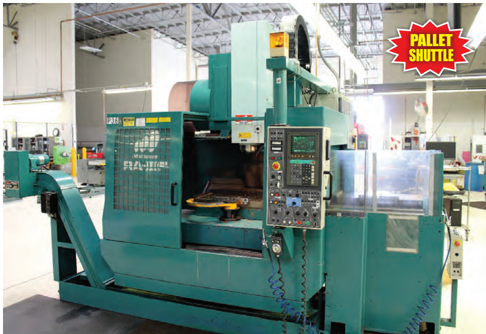
1998 MATSUURA MC-600 VF, YASNAC I-80 CNC CONTROL, 23" X 16" X 18", 8000 RPM SPINDLE, CAT 40 TAPER, 20 STATION ATC, 10 HP, S/N 980713232
