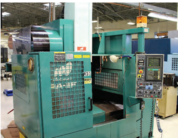
1996 MATSUURA RA-III-F, TWIN PALLET CHANGER, YASNAC MX3 CNC CONTROL, TRAVELS: 23" X 16" X 18", 6000 RPM SPINDLE, BT 40 TAPER, 20 STATION ATC, 15 HP, FLOOD COOLANT SYSTEM S/N 960912234
