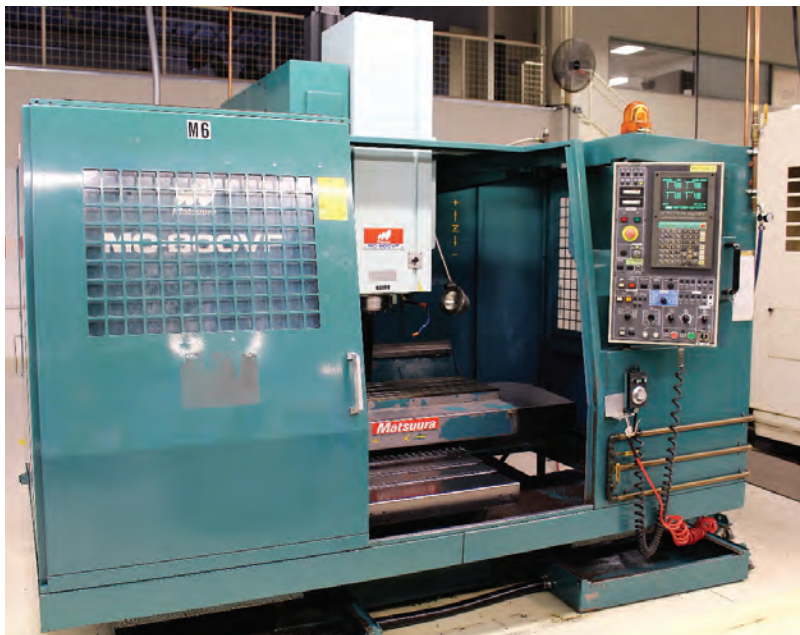
1993 MATSUURA MC-800 VF, YASNAC I-80 CNC CONTROL, TRAVELS: 32" X 17" X 19", 7000 RPM SPINDLE, CAT 40 TAPER, 30 STATION ATC, 10 HP, S/N 930710296
