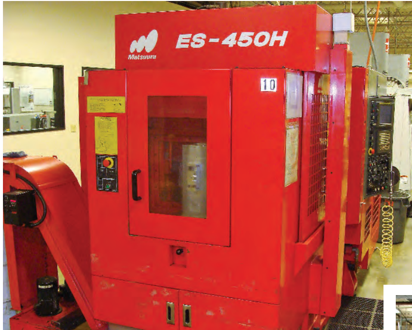
1998 MATSUURA ES-450H, 181-M FANUC CNC CONTROL TRAVELS: 17" X 15" X 15", TWIN PALLETS, 1 DEGREE INDEXING, HIGH TORQUE SPINDLE, BT 40 TAPER SPINDLE, 10000 RPM SPINDLE, 30 ATC, 10 HP, COOLANT, CHIP CONVEYOR, S/N 971112851
