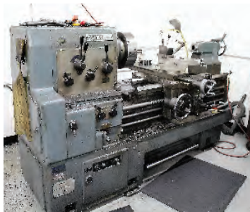
MORI SEIKI MODEL MH-1000G, 24" / 31" X 40" CG, 12" 3 JAW CHUCK, 20" 4 CHUCK, 3" HOLE, S/N 4217
