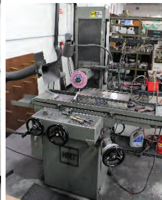
MITSUMI HIGH TEC, MSG-250 MH, 6" X 18" WALKER MAGNETIC CHUCK, MITUTOYO LINEAR SCALES, S/N 96066098
