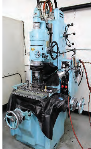
MOORE G-18, TABLE: 11" X 14", TRAVELS: 18" X 11", 225 RPM SPINDLE, S/N G-376, TOOLING, OAK CABINET, ROTARY TABLE
