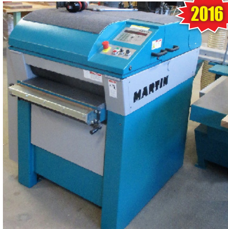
2015 MARTIN MODEL T-45, 630MM WIDTH, 2.8 TO 300MM THICKNESS, 1260MM TABLE LENGTH, S/N 539107
