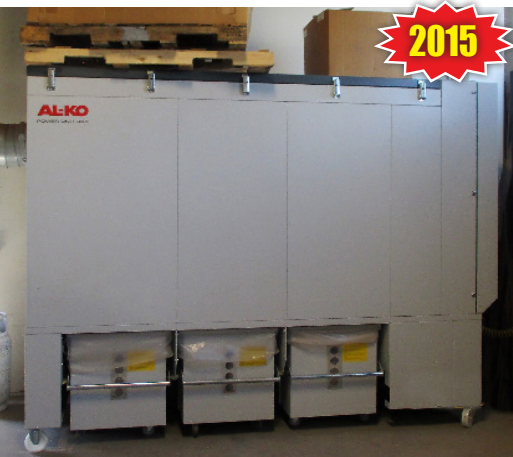
2015 AL-KO MODEL AP4 300P 3X220V, COMPRESSED AIR CLEANING, PRE-SEPARATOR, 3 DISPOSAL CONTAINERS 250 L EACH, INTEGRATED AUTOMATIC FIRE EXTINGUISHER
