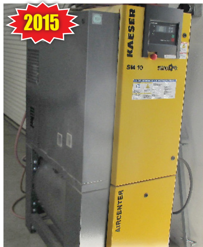
2015 KAESER MODEL SM-10, ROTARY AIR COMPRESSOR, 10 HP, S/N 1.8.8102.3
