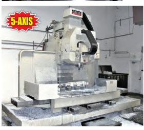
SNK FSP-80V TITANIUM MILLING MACHINING CENTER, FANUC 311A5 CTRL, 90.5" X 33" X 27.5", A & B AXIS +/- 30 DEGREES, 4000 RPM, 50 TAPER, 40 HP, 40 TOOL ATC, CHIP CONVEYER, INSTALLED NEW 12/2013 SERIAL NUMBER: 453227
