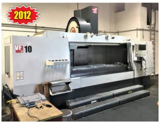
HAAS VF10/50, HAAS CTRL, 120" X 32" X 30", 50 TAPER, 7500 RPM SPINDLE, 30 HP SPINDLE, SIDE MOUNT 30 ATC, CHIP AUGER, NEW 3/2012 S/N: 1093175
