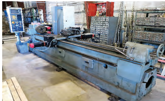
WANDERER, FANUC O-M CNC CONTROL, 3" HOLE THRU, 12" 3 JAW CHUCK, 6" X 120" CC
