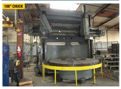
HENRY BROADBENT VERTICAL TURRET LATHE; 108" 4 Jaw Chuck; (2) Five Station Turrets; 70" Under Rail; 84" Swing; 40HP; Pendant Control
