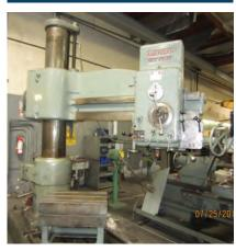
AMERICAN HOLE WIZARD RADIAL ARM DRILL; 13" Column x 60" Arm; w/ 20" x 30" x 10" Box Tbl.; 15-1200 RPM, Year 1964
