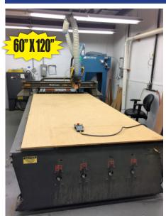
**MULTI CAM 3000 ROUTER, MODEL** 905-0059, 60" X 120" WORK AREA, **DUAL SERVO MOTORS ON GANTRY, VACUUM** PUMP, 8 HSK **TOOL HOLDERS, BRUSHLESS SER-VOS, 8 POSITION TOOL CHANGER,** 4,000-24,000 RPM, VACUUM **TABLE, MULTI-CAM EX HANDLE** CONTROL, S/N 900001781, **AIR FLOW DUST** COLLECTOR
