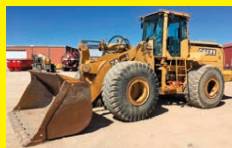
JOHN DEERE 744H SNDW744HX567548 John Deere diesel, EROPS, air, ride control, GP bucket, 26.5R25 rubber.
