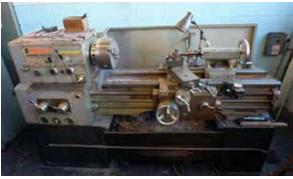
SELECT MACHINE TOOL 1640G GEARED HEAD GAP BED ENGINE LATHE, 16" SWING, 24" SWING IN GAP, 8" SWING OVER CROSS SLIDE, THREADING AND DIAL, TOOL POST, COOLANT SYSTEM, TRAV-A-DIAL GAUGE, STEADY REST
