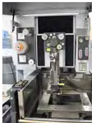
2015 SODICK SL400Q WITH LN2W CONTROL, LINEAR MOTOR HIGH PERFORMANCE WIRE EDM, 17" X 12.5" X 11", U AND V AXIS 6.10" X 6.10"
