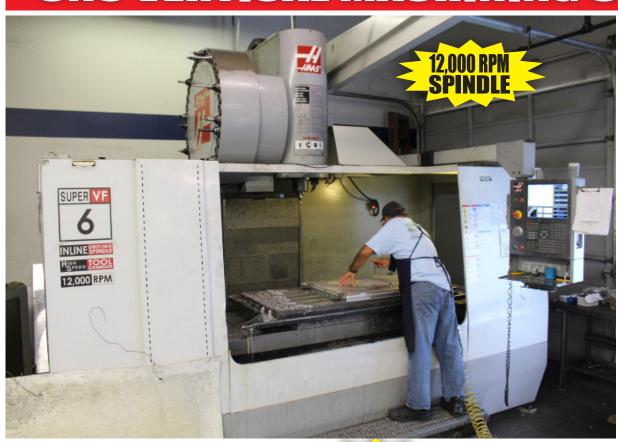
2008 HAAS VF-6SS, XYZ TRAVELS: 64" X 32" X 30", 12,000 RPM SPINDLE, 40 TAPER SPINDLE, 24 STATION SIDE MOUNT TOOL CHANGER, CHIP AUGER, COOLANT THRU SPINDLE, ZENON LIGHTING, INLINE DIRECT DRIVE, S/N 1063885
