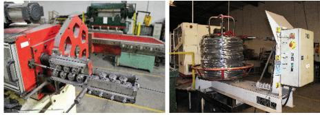
2001 LATOUR ROBOMAC MODEL 310 CNC 3D WIRE BENDERS; WIRE DIA. RANGE: .118" TO .393" (3 TO 10MM), FIVE AXIS, FORMING HEADS, FEED LENGTH UNLIMITED, (1) WITH REAR ROTATING STRAIGHTENING ATTACHMENT, DNC-800 CNC PROGRAMMABLE CONTROL, LATOUR MODEL D1000 MOTORIZED HORIZONTAL DECOILER; S/N 01-011-53
