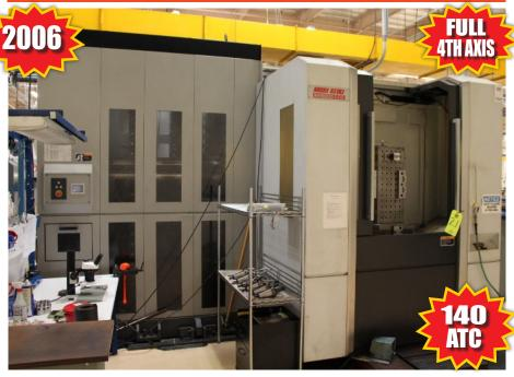
2006 MORI SEIKI NH5000 DCG HORIZONTAL MACHINING CENTER, MSX-70 III CNC CONTROL, FULL 4TH AXIS, XYZ TRAVEL AXIS: 28.74" X 28.74" X 32.67", 140 ATC, BT50 TAPER SPINDLE, 8,000 SPINDLE RPM, COOLANT THRU SPINDLE, RENISHAW PROBE, MOSNIC CHIP CONVEYOR, COOLJET SYSTEM, HIGH SPEED RAPID TRAVERSE, QUANTITY OF BT50 TAPER TOOL HOLDERS & COLLETS, VIDMAR 3-DRAWER TOOL CABINET W/ CONTENTS, 10-DRAWER TOOL CABINET W/ CONTENTS, S/N NH502F10108
