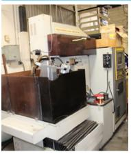
PRATT & WHITNEY TAPE CUT W2 WIRE TYPE, FANUC CNC CONTROL ELOX SINKER TYPE, FANUC CNC CONTROL
