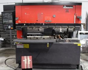
AMADA RG-80, 88 TON, TABLE LENGTH: 94.6", MAX. BENDING LENGTH: 98.7", DISTANCE BETWEEN UPRIGHTS: 80.8", THROAT DEPTH 15.76", NC9-EXII CNC CONTROL, BACK GAUGE SYSTEM, S/N 811695
