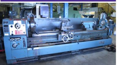
2006 KINGSTON HD 22120, 22" X 120" CC, 31" SWING IN GAP, 4" SPINDLE BORE, 1200 RPM, 10" CAPACITY STEADY REST WITH ROLLER JAWS, 12" BACK PLATE, 4-WAY TOOL POST, AUTO-MATIC LONGITUDINAL FEED STOP BAR, THREAD CHASING DIAL, LONGITUDINAL RAPID TRAVERSE, FOOT BRAKE SYSTEM, COOLANT SYSTEM WITH PUMP AND PIPING, FULL LENGTH SPLASH GUARD, DRO, S/N CH06907
