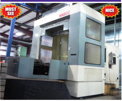
NIIGATA HN8OC, FANUC 15M CNC CONTROL, TRAVELS: 60" X 48" X 36", 31.5" X 31.5" DUAL PALLETS, AUTOMATIC PALLET CHANGER, COOLANT THRU SPINDLE, 40 HP, FULL 4TH AXIS, 60 ATC, 4,500 RPM, S/N 46250040
