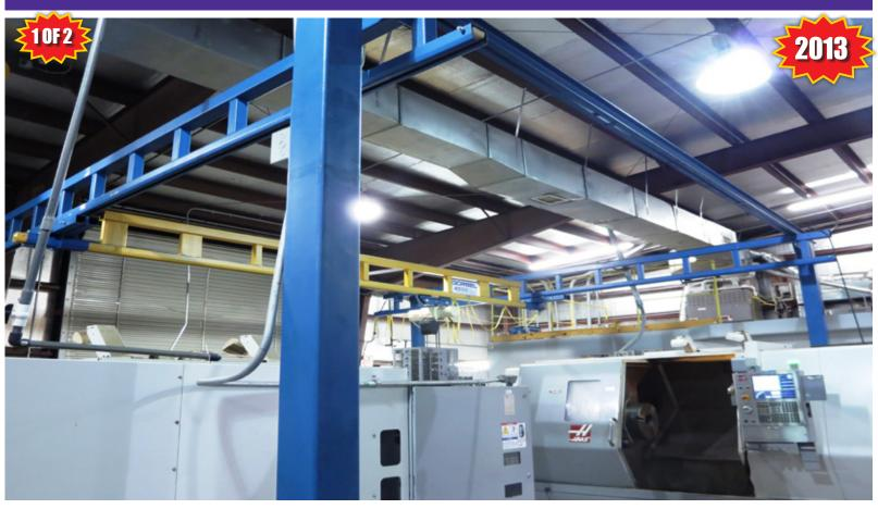
2013 GORBEL 4,000 LBS CAPACITY, BRIDGE WIDTH: 23', RUNWAY SERIES 4000: 50', COFFING 2 TON HOIST 2013 GORBEL 4,000 LBS CAPACITY, BRIDGE WIDTH: 23', RUNWAY SERIES 4000: 25', COFFING 2 TON HOIST
